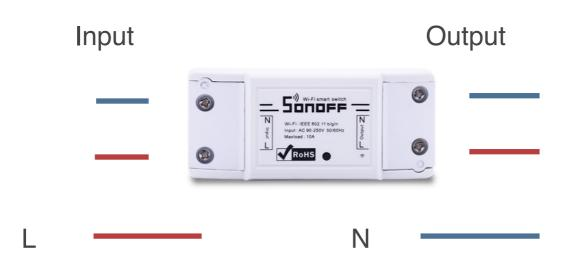
For the correct connection of the switch with the appliance, eg a bulb, it is necessary to use the connection as shown above. Connect phase and working conductor (L and N).
